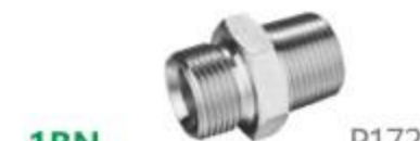
1BN P172 英管外螺纹60°内锥或六角端面用组合垫密封 美制布锥管外螺纹 BSP MALE DOUBLE USE FOR 60° CONE SEAT OR BONDED SEAL/NPT MALE
