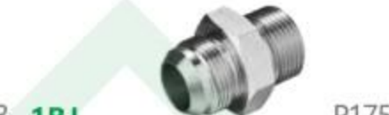
1BJ P175 英管外螺纹60°内锥或六角端面用组合垫密封/美制JIC外螺纹74°外锥 BSP MALE DOUBLE USE FOR 60° CONE/SEAT OR BONDED SEAL /JIC MALE 74°CONE
