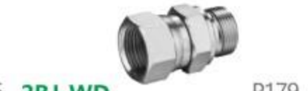
2BJ-WD P179 英管外螺纹胶垫密封/美制JIC内螺纹74°内锥 BSP MALE CAPTIVE SEAL / JIC FEMALE 74°SEAT
