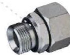
英管螺纹胶垫密封柱端 公制内螺纹24° 锥O形圈密封 BSPP THREAD WITH CAPTIVE SEAL METRIC FEMALE 24° CONE O-RING SEALING
