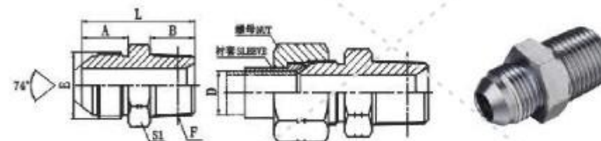
JIC外螺纹74° 外锥/ 布锥管外螺纹 JIC MALE 74° CONE / NPT MALE
