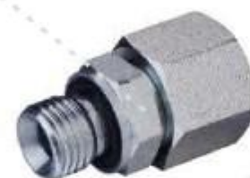
公制螺纹胶垫密封柱端/ 公制内螺纹24° 锥O形圈密封 METRIC THREAD WITH CAPTIVE SEAL/ METRIC FEMALE 24° CONE O-RING SEALING
